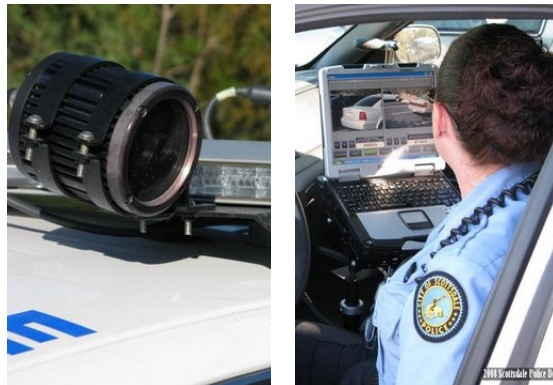
LPR camera & system
